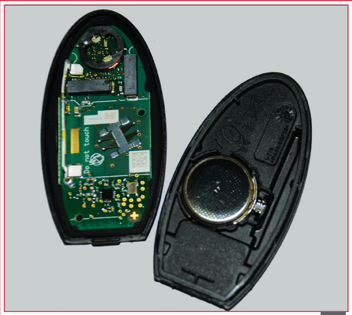
Continental Intelligent Key with the back removed
